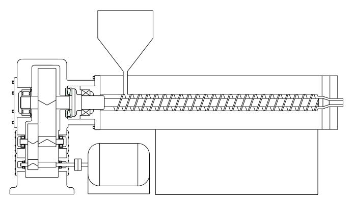
Tapered Thrust in Single Screw Extruder
