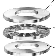
Bore is precision ground for a line to loose fit on shaft. The O.D. has a turned finish and is smaller than the housing plate's O.D.
