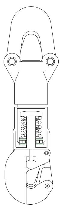
Hook Used On Drilling Rig
