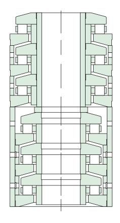
to each other, making the use of the tandem thrust bearing essential. Some twin screw extruder designs use eight stage tandem thrust bearings. We manufacture two, three, four, six and eight stage bearings in both inch and metric series. Bore sizes range from about 1 to 22 inches with corresponding outside diameters ranging from 3.5 to 42 inches. ROLLWAY® tandem thrust bearings are supplied to original equipment manufacturers and the aftermarket.
