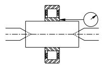
Outside Diameter of Outer Race - For determining outside diameter, use apparatus arranged for two-point measuring. Measure single diameters in at least three angular directions and two radial planes. In this manner D<sub>min</sub> and D<sub>max</sub> are established, from which the mean diameter is obtained by:
