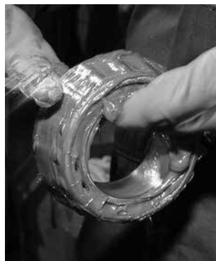
Fig. 51. Grease can easily be packed by hand.
